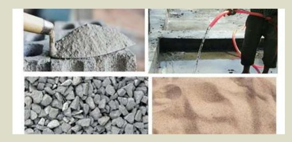
The most common materials are concrete, wood, metal, and stone. Concrete is a mixture of cement, water, and aggregate (sand and gravel). It is widely used for foundations, walls, floors, and driveways. Wood is also a popular construction material.
