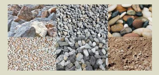
The aggregate gives volume, stability, resistance to wear or erosion, and other desired physical properties to the finished product. Commonly used aggregates include sand, crushed or broken stone, gravel (pebbles), broken blast-furnace slag, boiler ashes (clinkers), burned shale, and burned clay.
